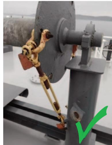
(Left) Showing mechanically secured winch reel.
