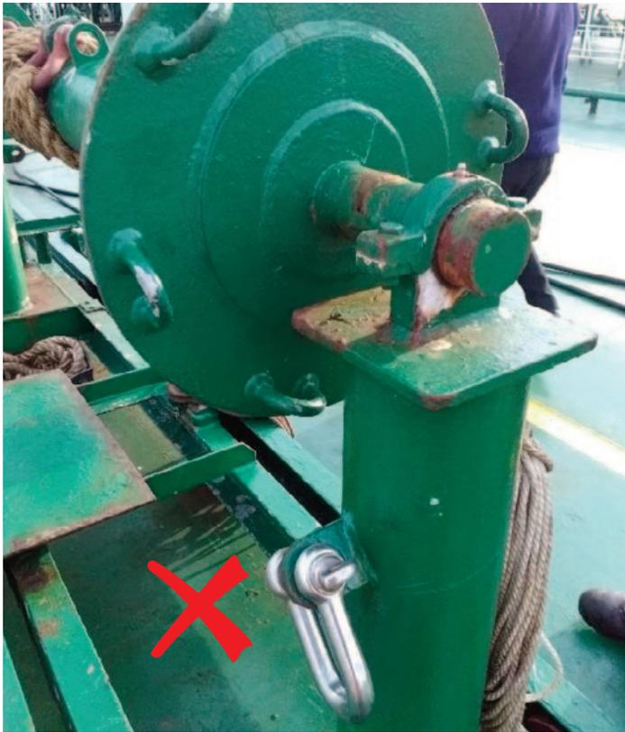
This example shows a winch reel that has not been mechanically secured.
