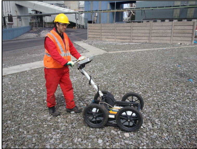
Plate 3 – MALA RAMAC 250MHz GPR cart system (library photograph)
