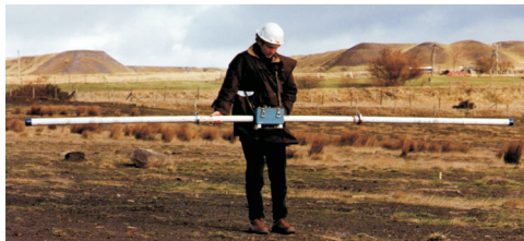
EM-31 (Exploration depth ~3 to 5m)
