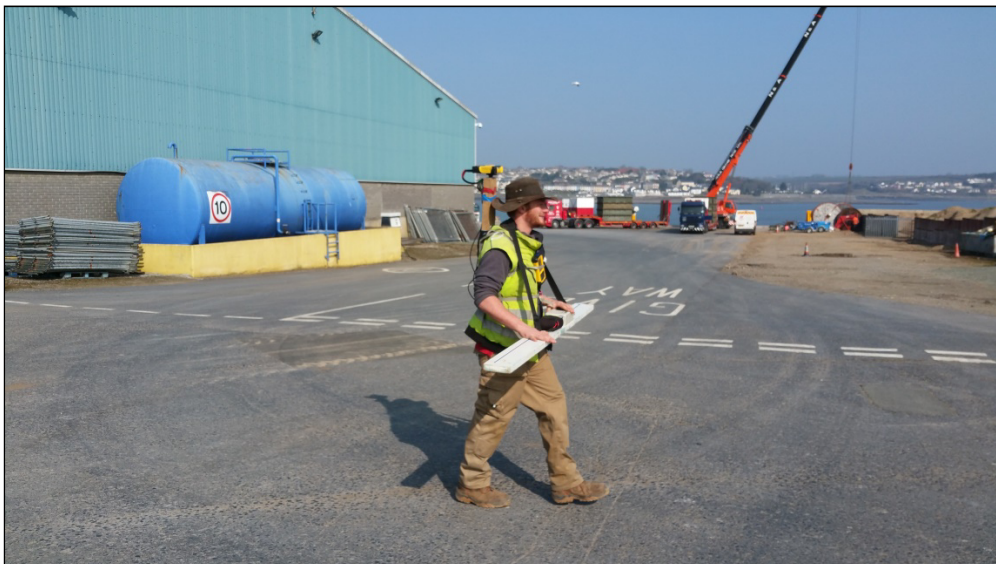
Plate 2 - Geophex GEM-2 with Trimble DGPS positioning being used at the site
