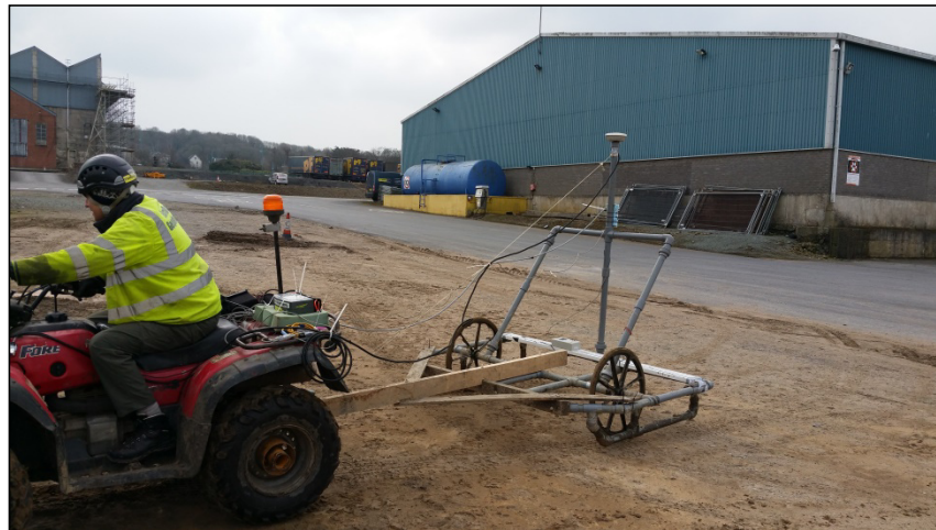
Plate 1 – Towed G858 Magnetic Gradiometer being used at the site
