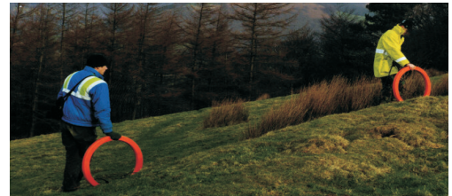
EM-34 (Exploration depth ~7.5 to 60m)
