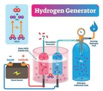
Using fuel cell technology, we can reverse the electrolysis process and generate electricity, from the stored hydrogen's repairing with oxygen, and the only by-product is water. This is how most hydrogenfuelled electric vehicles operate. This chemically elementary process could hold the key to helping us smooth the unavoidable peaks and troughs of renewable energy generation that relies on sun, wind, wave or tide.
