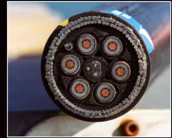
↑ Wired - an armoured submarine cable takes generated electricity back to land and transmits control data through hair-thin fibre optic cables
