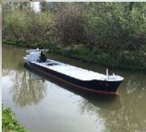
↑ We’re going to need a bigger boat - As part of her training Gillian underwent ‘manned’ model exercises in scaled down models that handle just like real ships.
