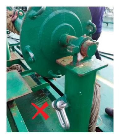
This example shows a winch reel that has not been mechanically secured.
