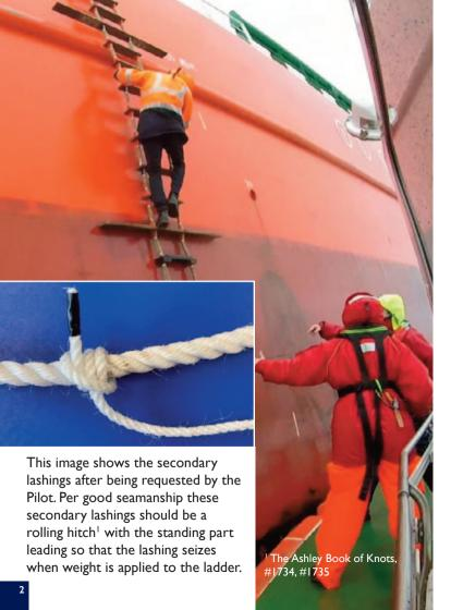
Milford Haven will not accept pilot ladders secured around railings or hand rails.
